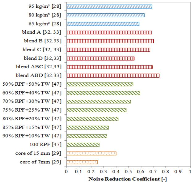
**Figure 4.** Noise reduction coefficient for same examined composite materials
