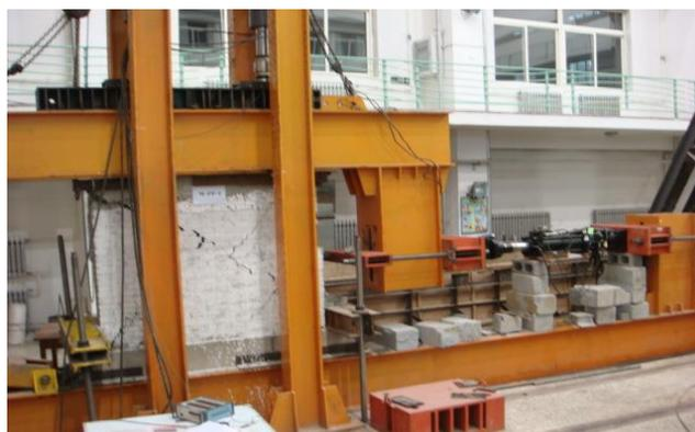
Fig.1. Picture of Loading Devices of The Test
