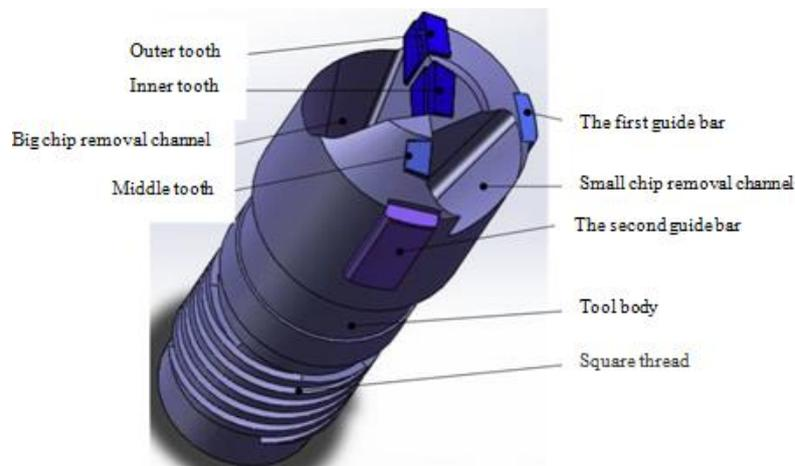
Fig.1. Graphic model of staggered teeth BTA drill
