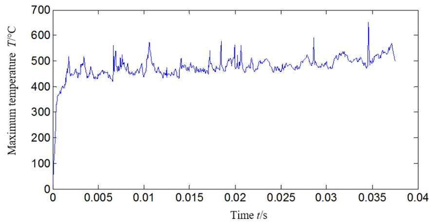
Fig.7. The maximum workpiece temperature vs. time  $t$
