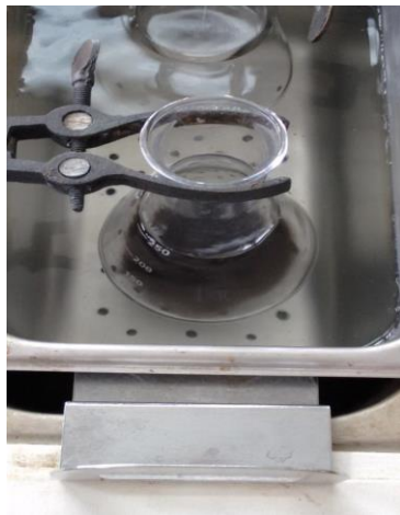
Sonication process of CuO-Water nanofluids
