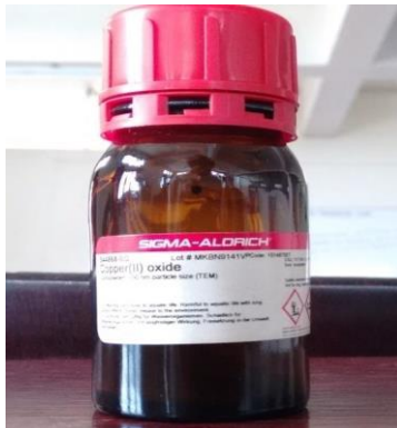
Copper oxide nanoparticles of size <50nm
