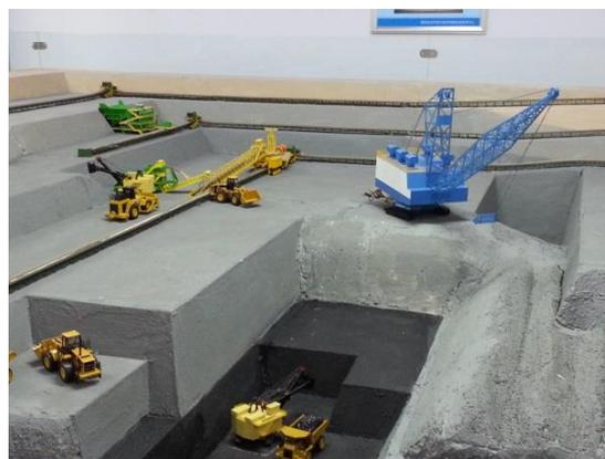
Fig. 1a. Model of high bench slope and dragline offset
