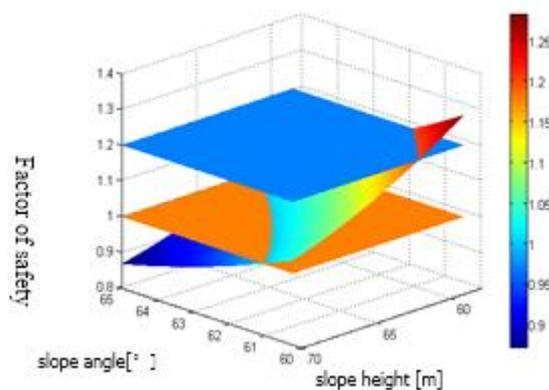
Fig.9. 3D curve graphic spitting the relationship between factor of safety, slope heights and angles with influence of blasting
