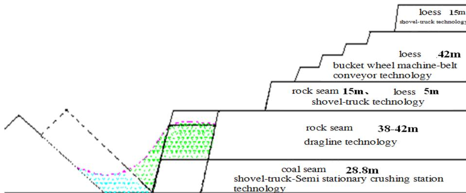
Fig. 3. Schematic diagram of mining technology section in West area
