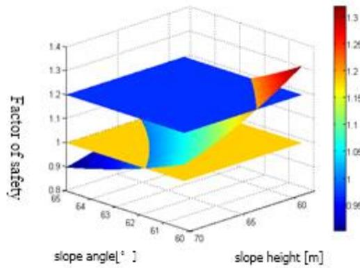
Fig.10. 3D curve graphic signifying the relationship between factor of safety, slope heights and angles with influence of ground water
