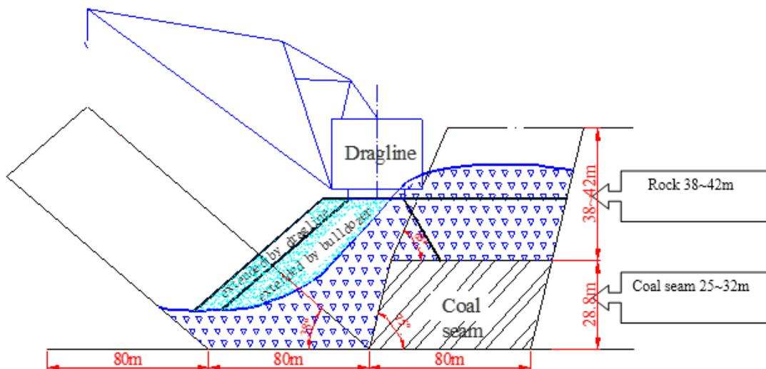
Fig. 1b. Sketch of dragline work on the high rock bench
