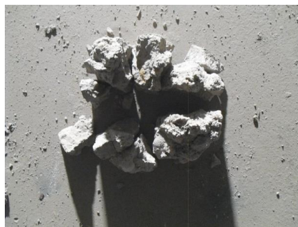
Fig. 10. Radial fracture of experiment 3.
