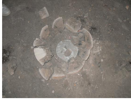
Fig. 11. Radial fracture of experiment 4.
