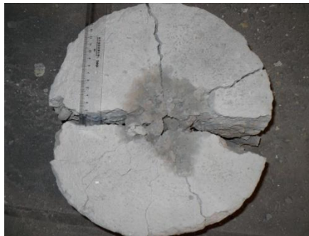
Fig. 12. Splitting effect of experiment 5.
