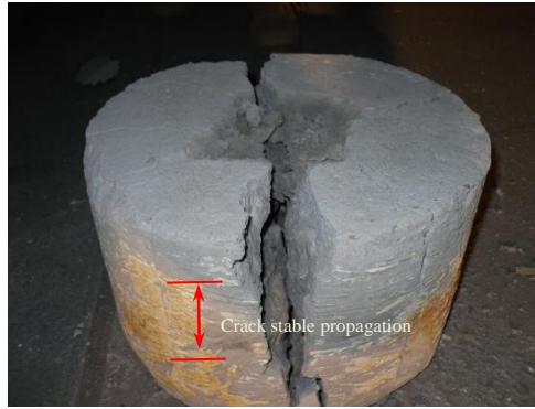
Fig. 13. Splitting crack propagation of experiment
