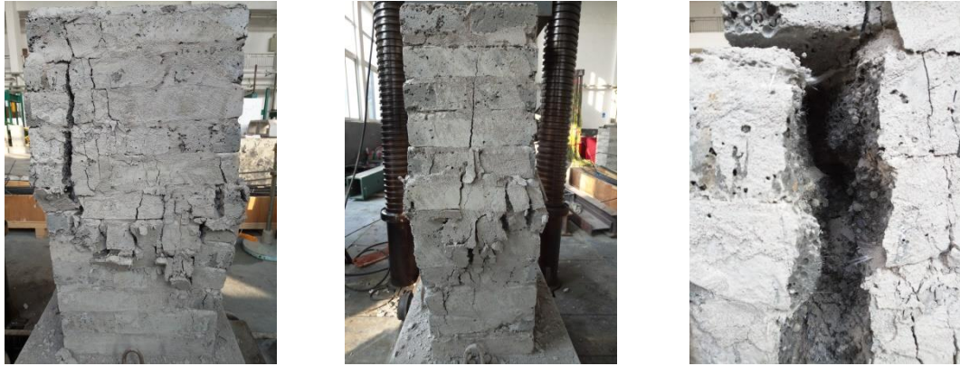
Fig.4. Typical failure modes of specimens
