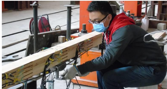
Fig.7. Pre-stress control of pre-stressed glue-lumber beam
