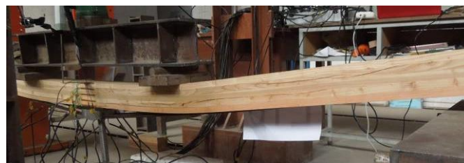
Fig.5. Plastic deformation of the beam
