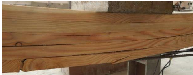
(c) Failure mode of beam L_{A1-6}
