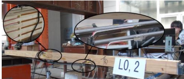
Fig.4. The illustration of strain gauge
