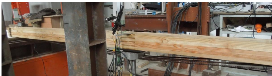
Fig.3. Pre-stressed glue-lumber beam
