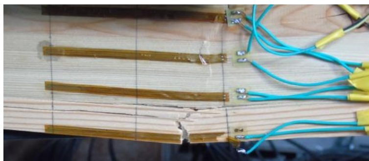
(b) Tension failure of the beam bottom
