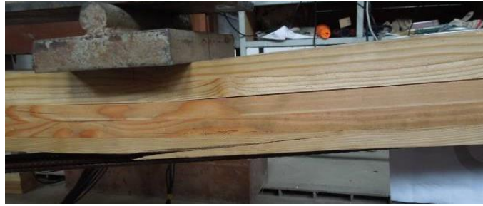
(a) Failure mode of beam L_{A1-2}
