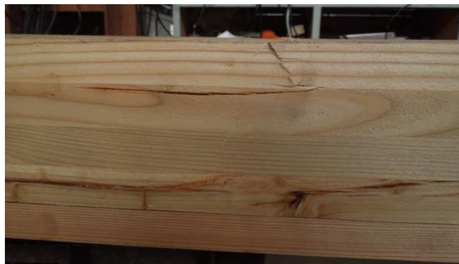
(a) Wrinkles on the side surface of three dividing points
