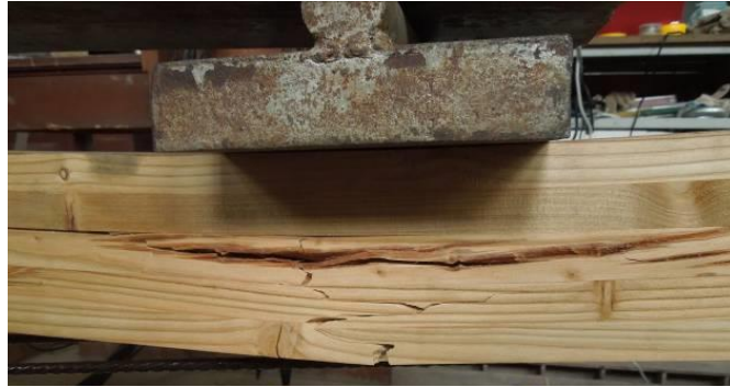
(b) Failure mode of beam L_{A1-4}
