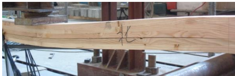
(a) Glue failure of the laminate
