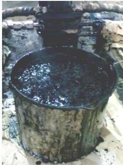
Fig.7 The test of asphalt foaming
