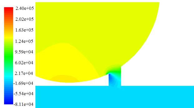
Fig.5 Pressure nephogram of foamed asphalt outlet
