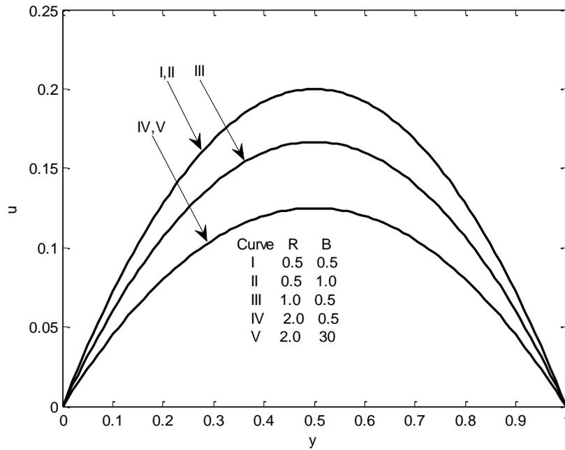
**Fig 5: Velocity profiles showing effect of  $R, B$  ( $S = 0, K_c = 0$ ) for  $m = m_1 = 1$ .**
