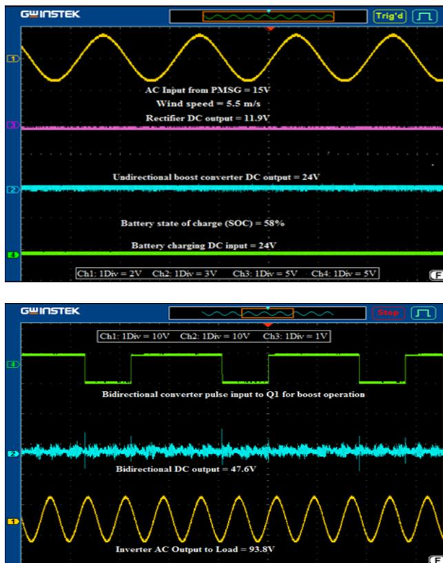
Figure 10. Hardware output result
