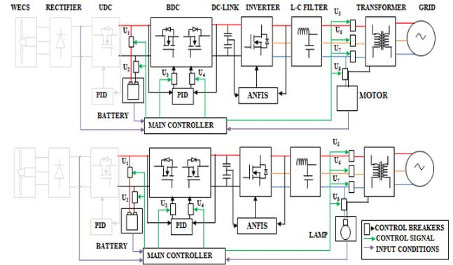
Figure 6. Grid power storage-load mode
