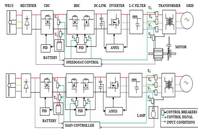
Figure 1. Wind energy conversion system with linear and non-linear load block diagram
