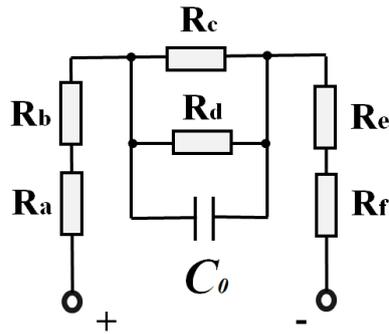
Fig.2. Electro-osmosis Equivalent Circuit Diagram
