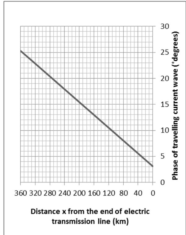
**Graph 1.** Magnitude (intensity) and phase (angle) of current travelling wave from the beginning towards the end of line ie. the direction the travelling wave moves (direction right to left of electric power transmission line of figure 1)
