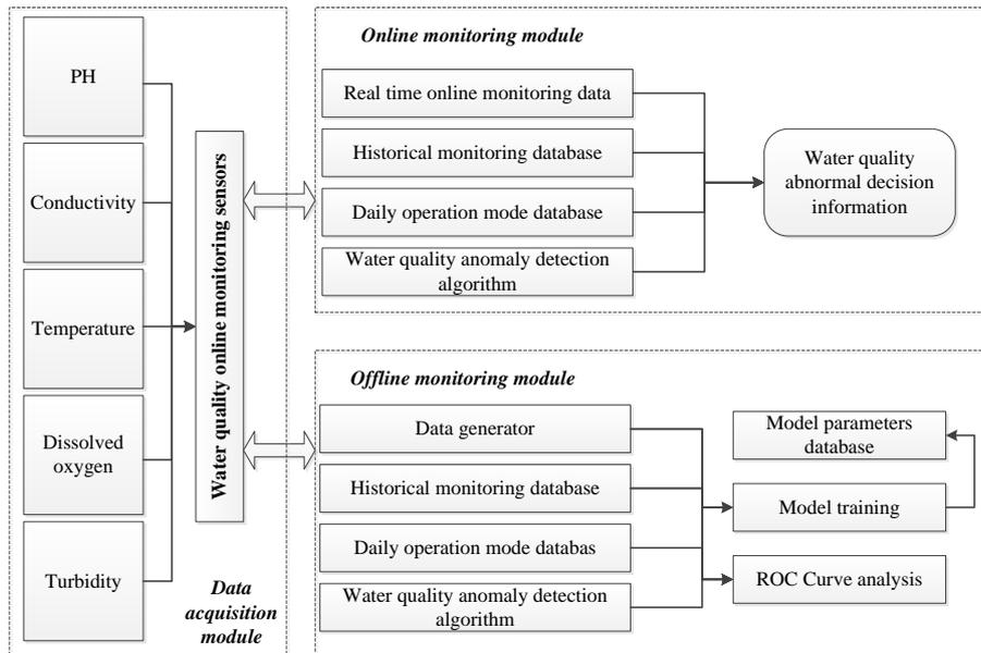
Fig.2. Framework of the water quality monitoring system
