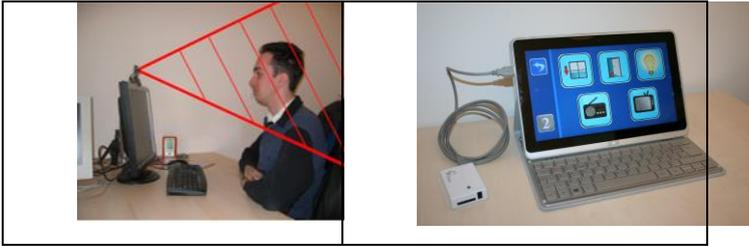
Fig 1: Installation of the Head Pilot on a desktop PC and field of action of the webcam for the analysis of the movements of the head (left), (right) coupling with Pictocom software to control home.
