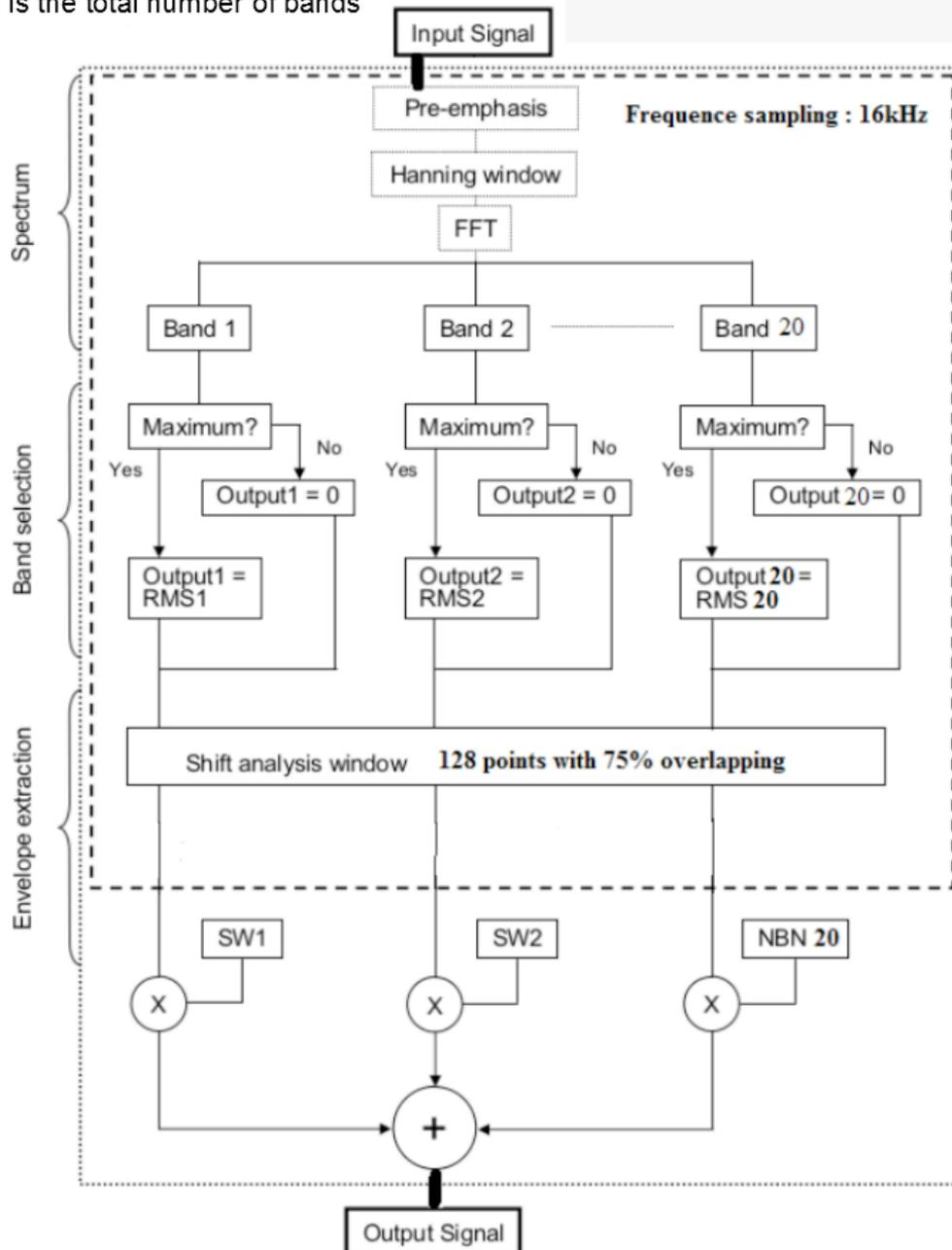
Fig. 2. Representation of cochlear implant coding
