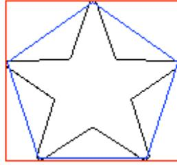
Fig.4. Representation of the convex hull (blue line) and bounding box (red line).
