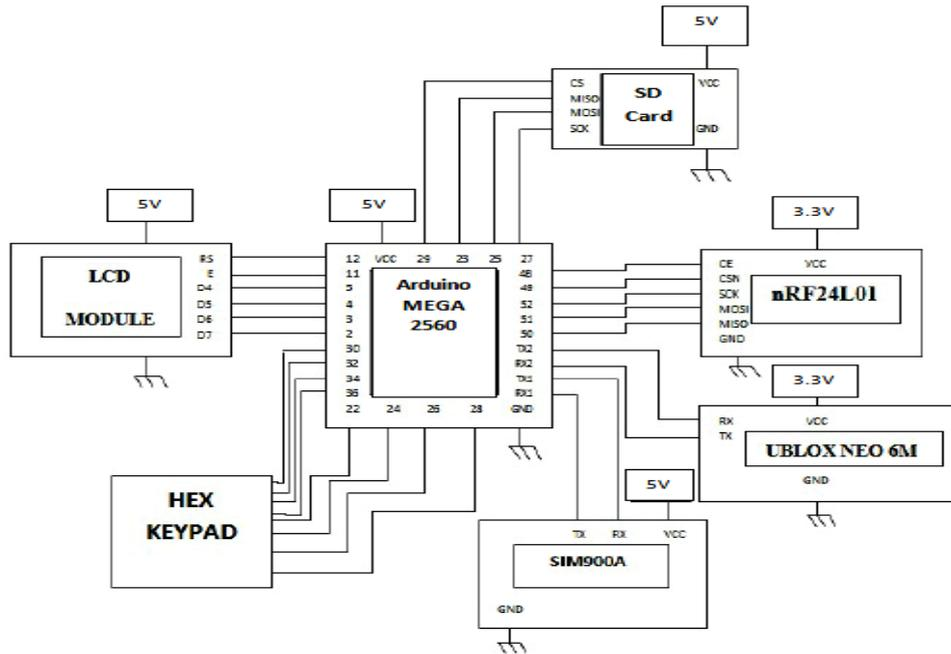
Fig.4. Circuit diagram of receiver section
