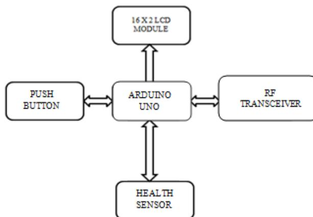
Fig.1. Block diagram of transmitter section
