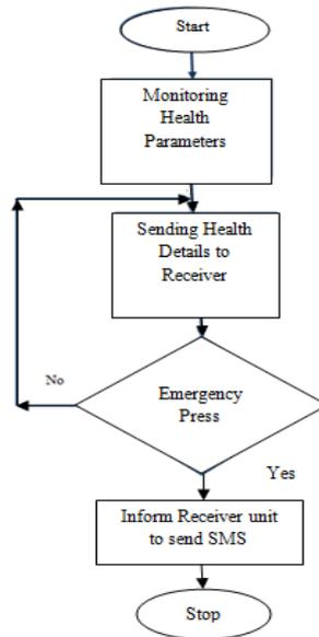
Fig.5. Flow chart of Transmitter Section
