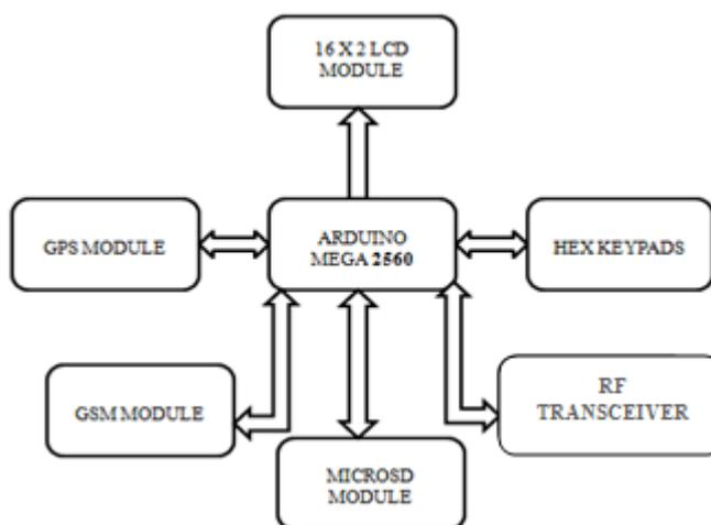
Fig.2. Block diagram of receiver section
