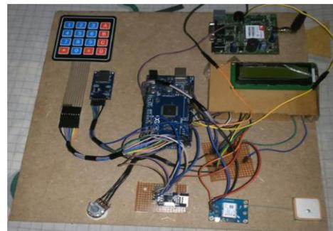
Fig 7: Hardware model of Transmitter Section and receiver Section
