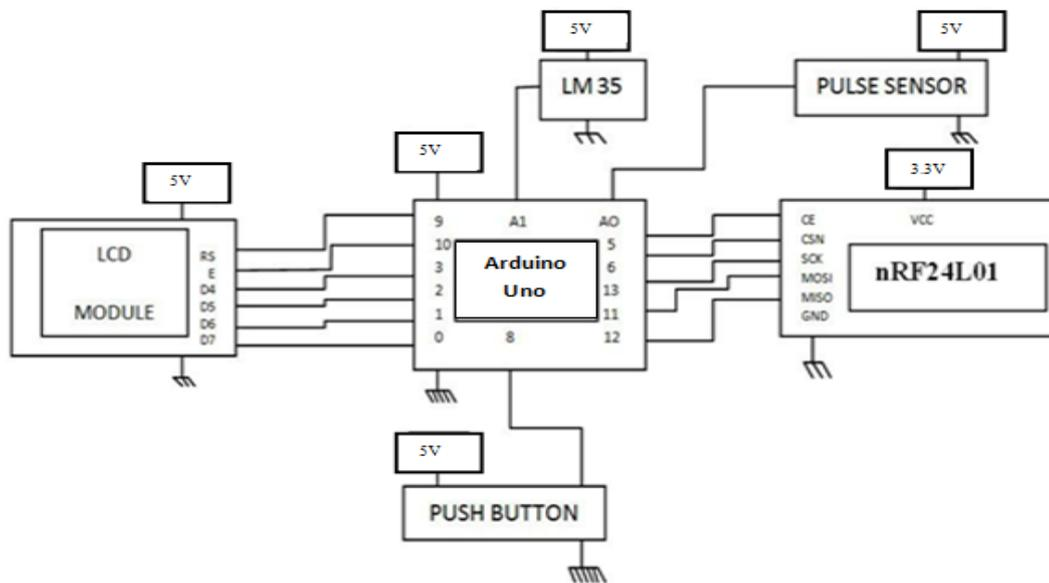
Fig.3. Circuit diagram of transmitter section
