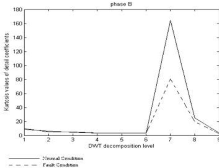
Fig.4. Kurtosis Values of Detail Coefficients for Phase B Current Plotted with Respect to DWT Decomposition Level
