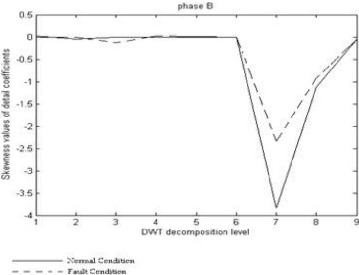
Fig.8. Skewness Values of Detail Coefficients for Phase B Current Plotted with Respect to DWT Decomposition Level
