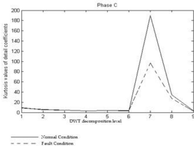
Fig.5. Kurtosis Values of Detail Coefficients for Phase C Current Plotted with Respect to DWT Decomposition Level
