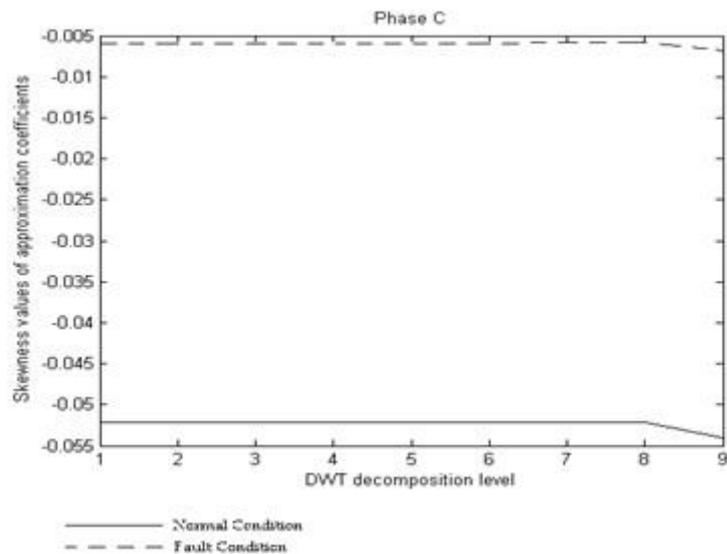
Fig.7. Skewness Values of Approximate Coefficients for Phase C Current Plotted with Respect to DWT Decomposition Level
