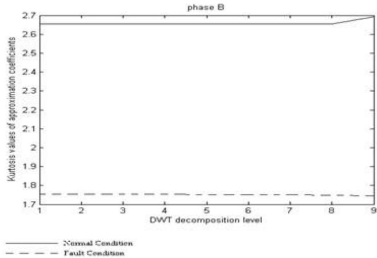
Fig.2. Kurtosis Values of Approximate Coefficients for Phase B Current Plotted with Respect to DWT Decomposition Level
