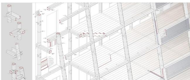
**Figure 2.** Kit overlaid to the existing building, with focus on the connections of the assembled profiles [25]
