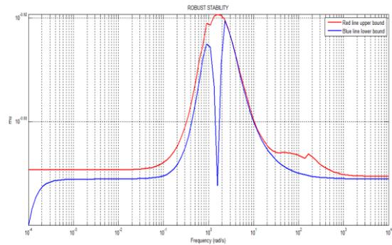
**Figure 12.** Robust stability test BLDC motor with  $H_\infty$  controller
