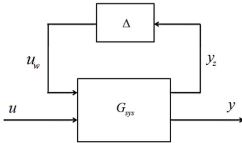
**Figure 5.** Upper LFT representation of the linear dynamical system
