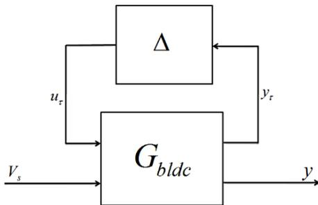
Figure 8. Upper LFT representation of BLDC motor
