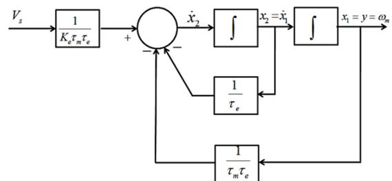
**Figure 6.** The block diagram representation of BLDC motor
