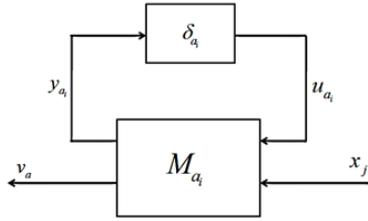
**Figure 2.** Representation of uncertain parameter  $\delta_{\beta_i}$  in upper LFT framework
