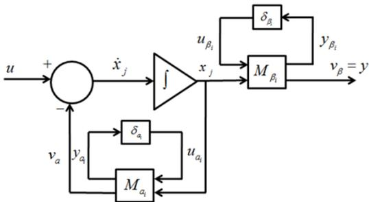
**Figure 4.** Block diagram representation with uncertain parameters
