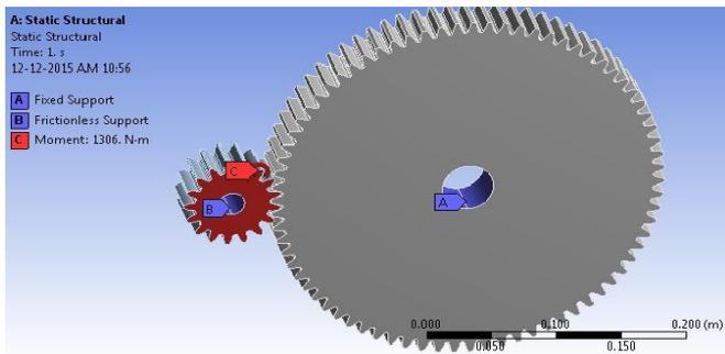
**Figure 2.** Boundary conditions for present analysis on spur gear pair
