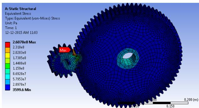
**Figure 3.** Bending stress distribution for steel C45 made gear pair
