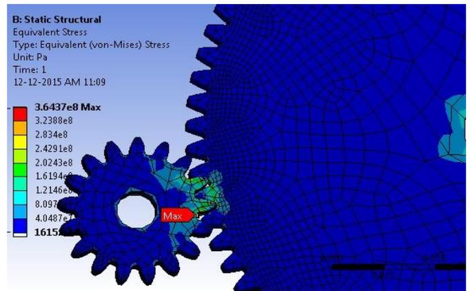
**Figure 4.** Bending stress distribution for HDPE made gear pair
