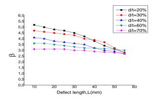
Figure 6. Effect of peak length L on reliability index  $\beta$
