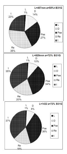
Figure 8. Distribution of reliability parameters depending on the model B31G
