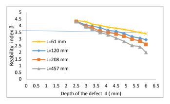
Figure 7. Variation of reliability  $\beta$  by different depth d with B31G
