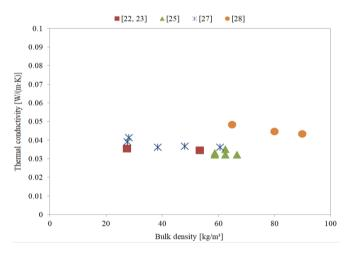
Figure 2. Thermal conductivity versus bulk density for insulating mats
