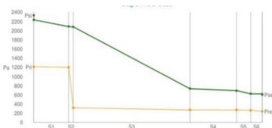
**Figure 10.** Diagram of Glaser for wood cover
