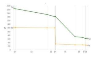
Figure 11. Diagram of Glaser for brick and concrete cover
