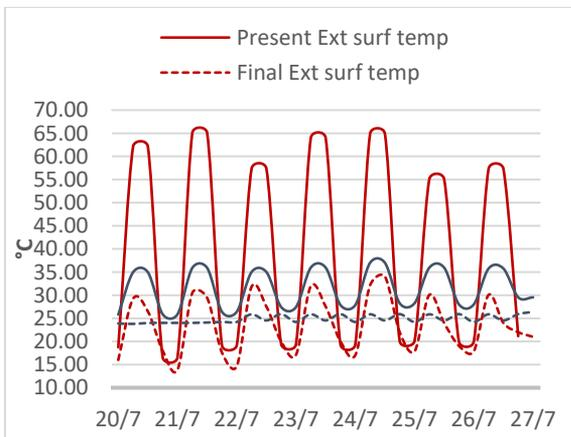
**Figure 13.** Temperature trend before and after cool material installation
