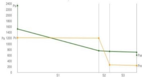
**Figure 4.** Diagram of Glaser for wood cover
