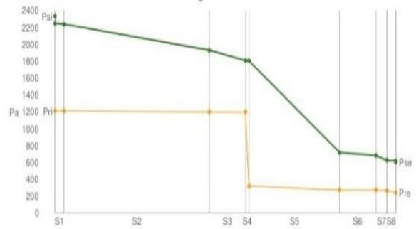
**Figure 11.** Diagram of Glaser for brick and concrete cover
