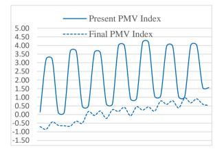
Figure 14. PMV index before and after cool material installation
