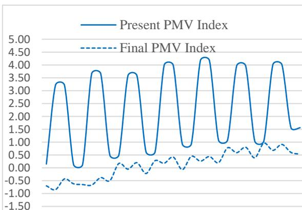
**Figure 14.** PMV index before and after cool material installation
