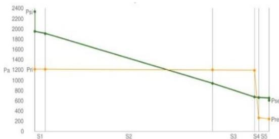
**Figure 5.** Diagram of Glaser for brick and concrete cover
