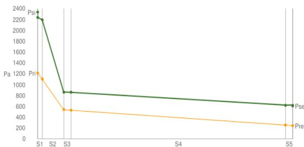
**Figure 9.** Diagram of Glaser of vertical walls
