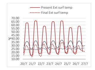
Figure 13. Temperature trend before and after cool material installation
