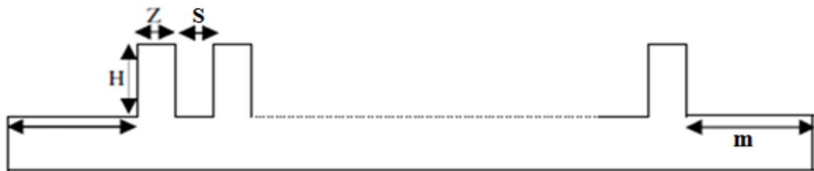
Fig.2. Arrangements of Rectangular Pin fin
