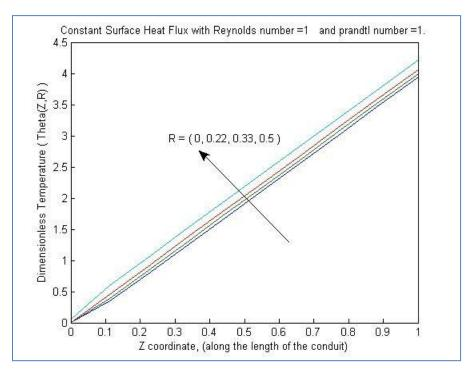
Fig. 5. Dimensionless temperature profile in entrance region for constant surface heat flux along
