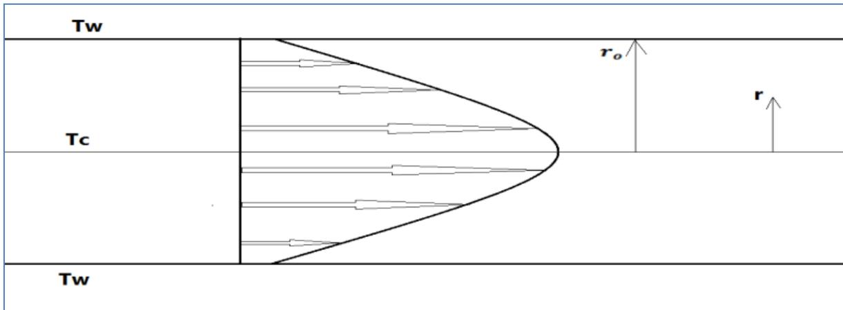
Fig. 3. Schematic diagram represents the temperature profile through the fully developed region inside the conduit
