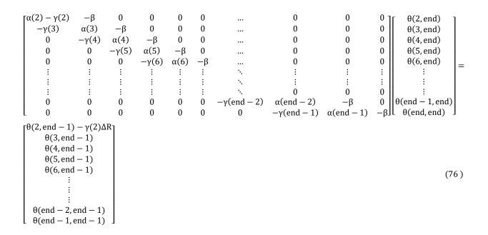
Each of these matrices equations (74-76) were solved to find the unknown elements of the  $\theta$  matrix. A program was built by using Matlab software, to describe the temperature variation at all points inside the conduit, such as it was illustrated in the matrix (77) below.
