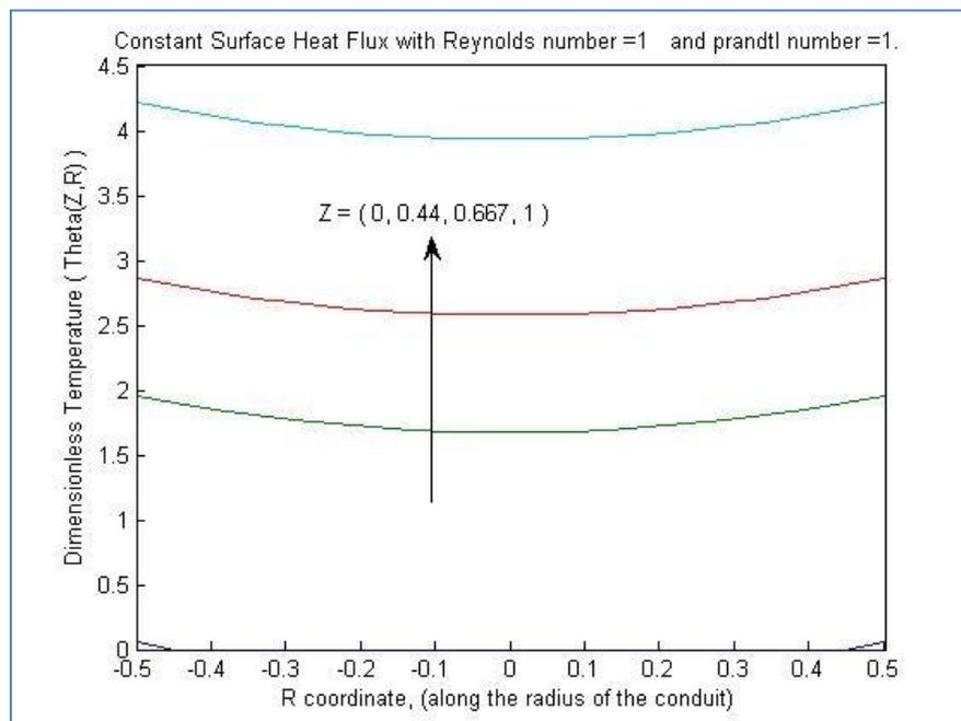
Fig. 6. Dimensionless temperature profile in entrance region for constant surface heat flux with radius of the conduit.
