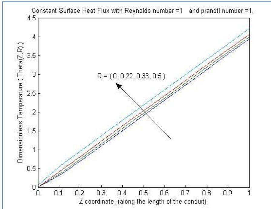
Fig. 5. Dimensionless temperature profile in entrance region for constant surface heat flux along the conduit
