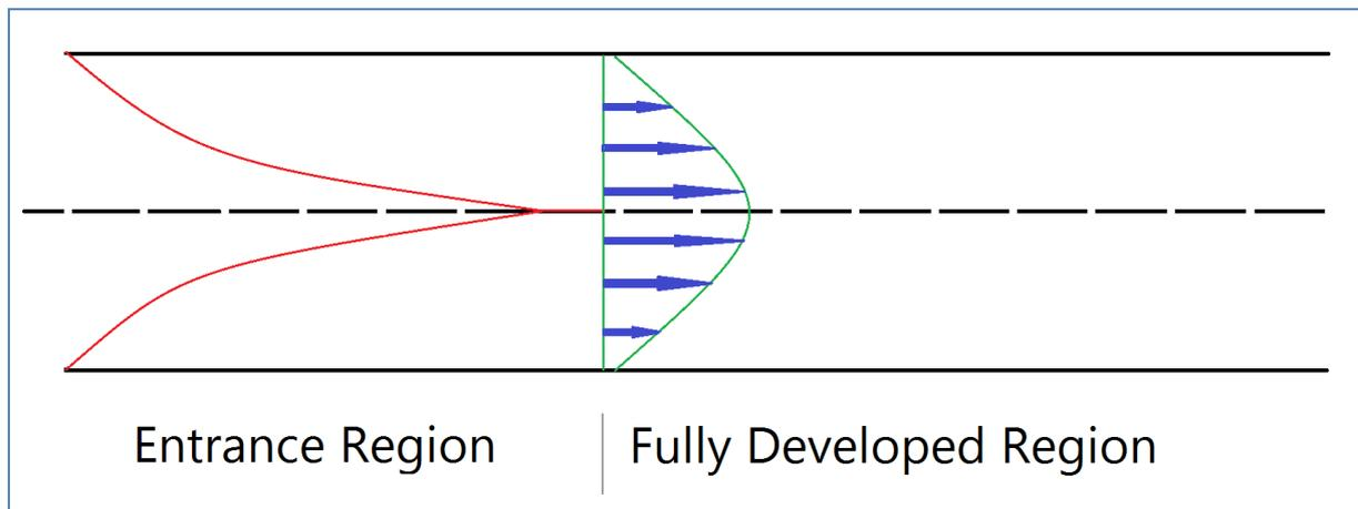
Fig. 2. Schematic diagram represents thermal entrance region inside the conduit
