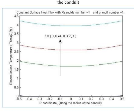
Fig. 6. Dimensionless temperature profile in entrance region for constant surface heat flux with radius of the conduit.
