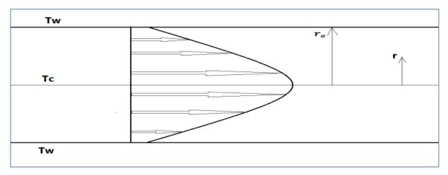
Fig. 3. Schematic diagram represents the temperature profile through the fully developed region inside the conduit
