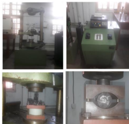
Fig.3. Laboratory testing for determination of UCS and tensile strength
