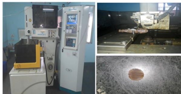
Fig.4. Roadheader conical picks cutting by EDM machine and size of 6/10 mm picks for SEM analysis.
