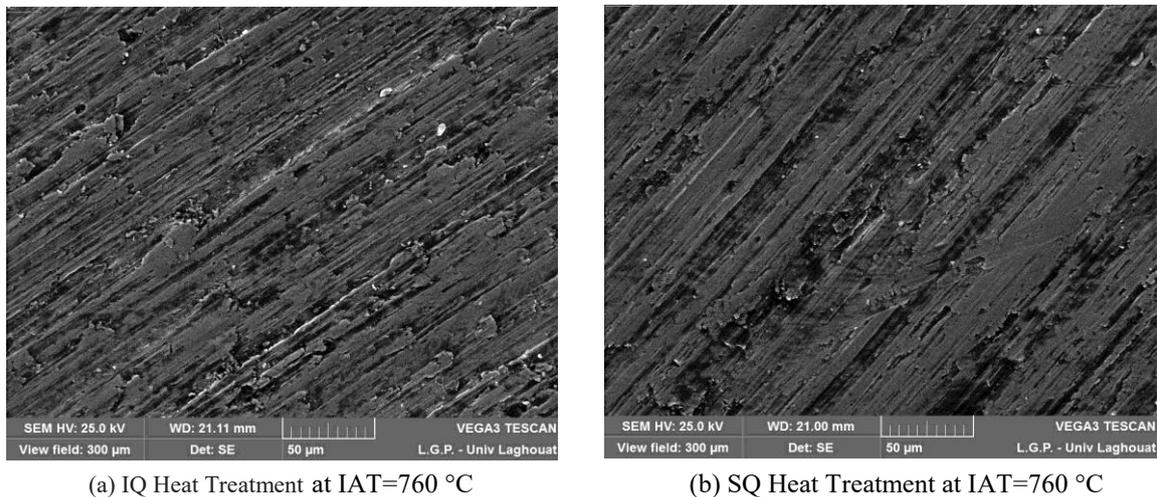
Fig.6. Abraded surface morphologies of DP steel tested at a load of 3 Kg
