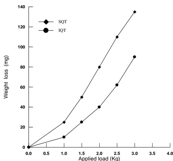
Fig.3. The Influence of the Type of Heat Treatment (IQT) and (SQT) on the Wear Abrasive Resistance as a Function of Applied Load for the Same IAT = 800 °C.
