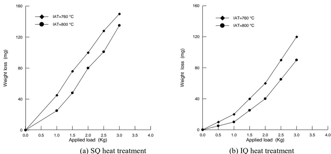
Fig.4. the effect of Intercritical Annealing Temperature on the abrasive wear resistance of various heat treatment samples as a function of applied load
