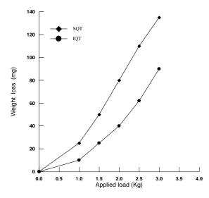
Fig.3. The Influence of the Type of Heat Treatment (IQT) and (SQT) on the Wear Abrasive Resistance as a Function of Applied Load for the Same IAT = 800 °C.
