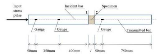
Fig.1. Schematic Diagram of Simplified SHPB Test
