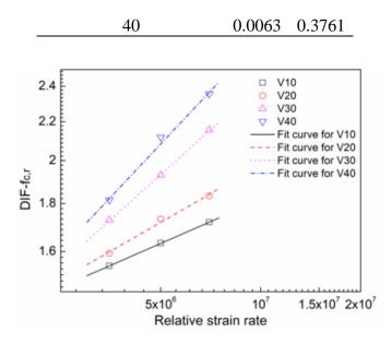
Fig.10. Variation of DIF- $f_{c,r}$  with relative strain rate
