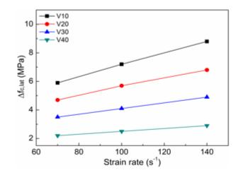
Fig. 4 Variation of  $\Delta_{fc,lat}$  with strain rate
