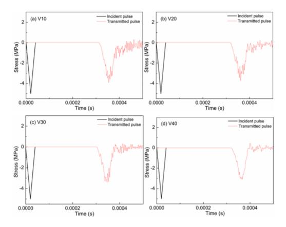
Fig.12. Transmitted stress pulse for stress wave T<sub>40</sub>F<sub>5</sub> through pressure bar1
