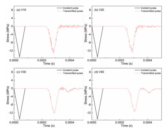
Fig.16. Transmitted stress pulse for stress wave T<sub>80</sub>F<sub>15</sub> through pressure bar2
