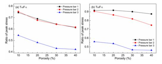
Fig.19. Ratio of transmitted peak stress of  $T_{40}F_{15}$  and  $T_{80}F_{15}$
