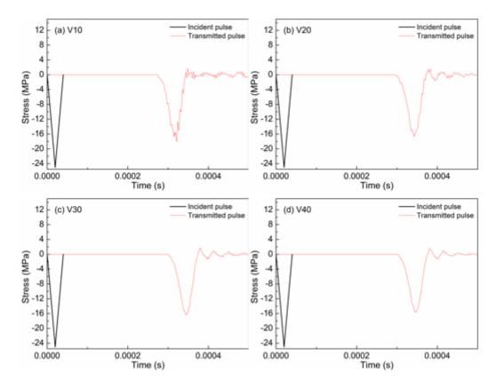
Fig.14. Transmitted stress pulse for stress wave T<sub>40</sub>F<sub>25</sub> through pressure bar1
