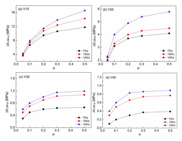
Fig.8. Variation of  $\Delta f_{c,lat-\mu}$  with friction coefficient
