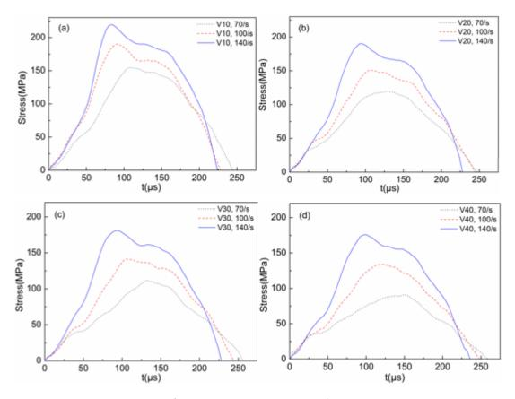
Fig.3. Input Stress Wave Pulses
