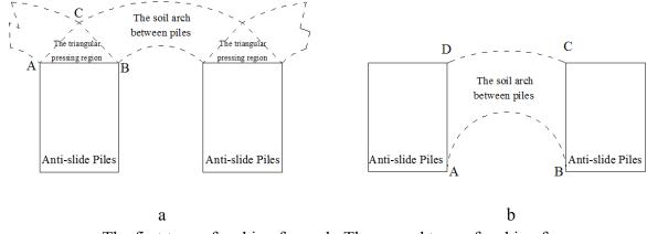
a: The first type of arching from b: The second type of arching form Fig. 2. Sketch Map of Two Types of Arching Forms of Rectangular Anti-slide Piles)
