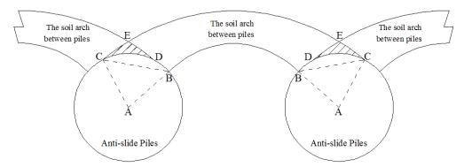
Fig.4. Sketch Map of the Arching Form of Mechanical Rotary Bored Anti-slide Pile
