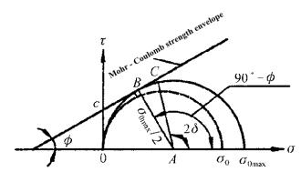
Fig.6. Unidirectional Pressed Mohr's Circle and Strength Criterion
