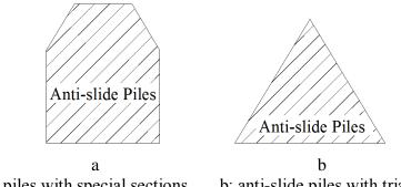
a: anti-slide piles with special sections b: anti-slide piles with triangular section Fig.1. Sketch Map of Anti-slide Piles with Other Section Types
