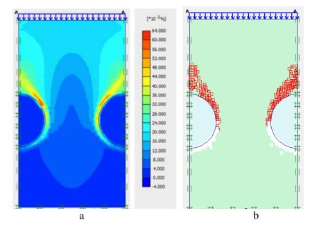
a:Cloud Picture of Shear Stress b:Sketch Map of Plasticity Point Fig.8. Sketch Map of Numerical Simulation Results
