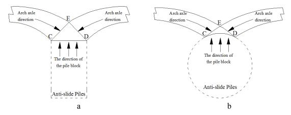
a: rectangular anti-slide pile b: mechanical rotary bored anti-slide pile Fig.3. Sketch Map of the Triangular Pressure-bearing Zone of Two Types of Anti-slide Piles
