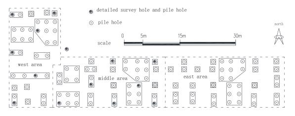
Fig.2. Floor plan for the pile foundation
