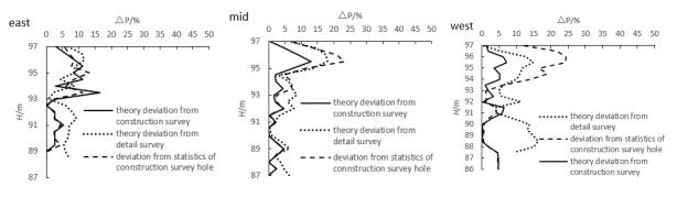
Fig.5. Rock embedding probability error curves of pile groups
