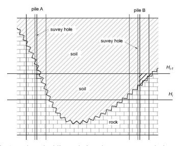
Fig.1. rock-embedding relations between survey hole and pile
