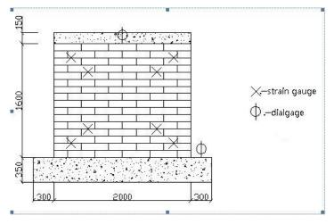
Fig.2. Floor Plan of Instrument and Strain Gauge
