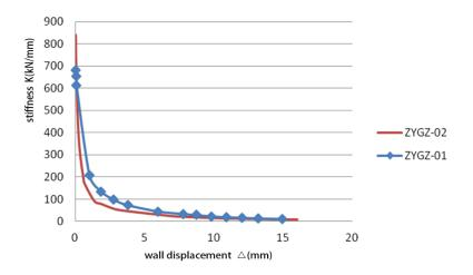
Fig.8. Stiffness Degradation Curves of Specimen
