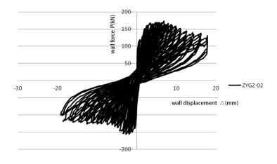
Fig.6. Hysteresis Curve of Specimen ZYGZ-02
