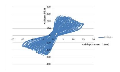
Fig. 5. Hysteresis Curve of Specimen ZYGZ-01
