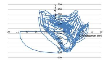
Fig.4. Strain-displacement Curve of Steel Bar in Specimens
