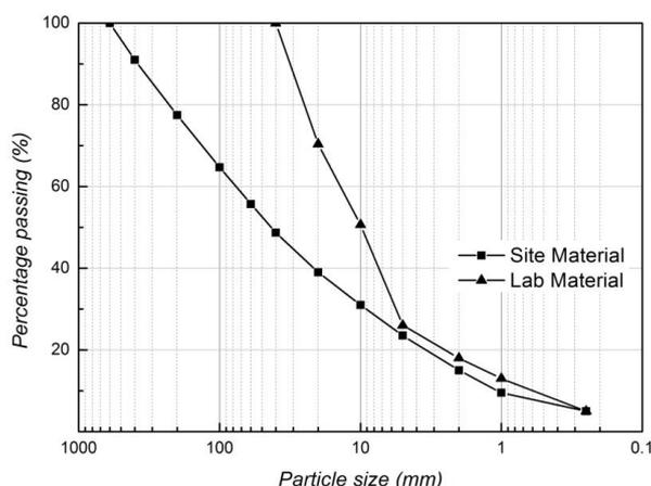
Fig.1. Grain-size distribution curve of the test material
