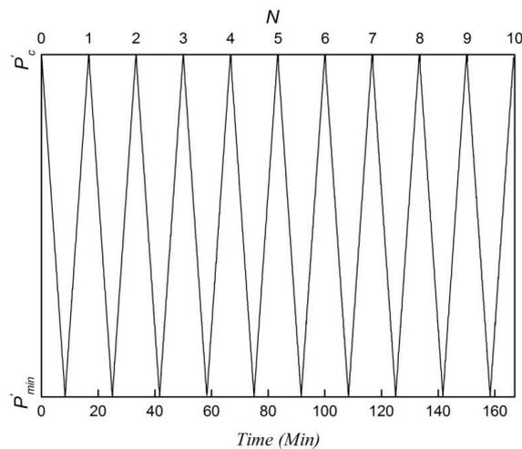
Fig. 2. Revolution of spherical stress with time/cyclic number
