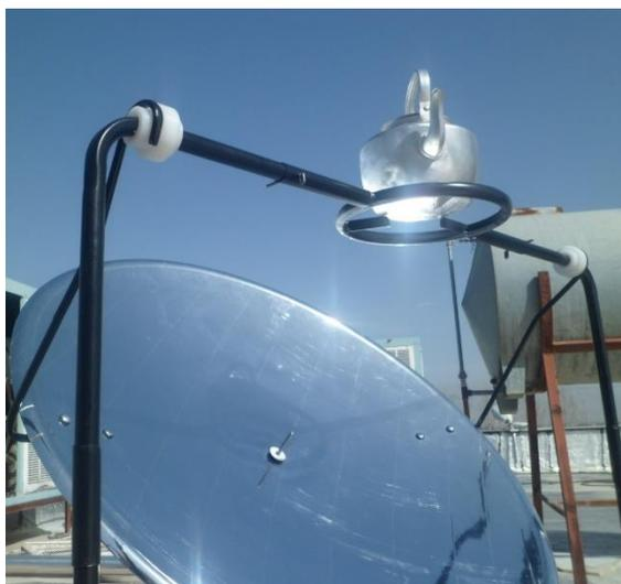
Fig.1. Photograph of the Solar Cooker.
