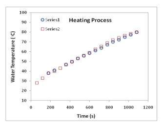
Fig.3. Water Temperature Variation During the Heating Process.
