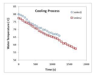
Fig.4. Water Temperature Variation During the Cooling Process.
