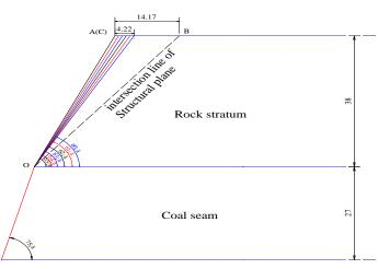
Fig. 5. Typical section of slope profile
