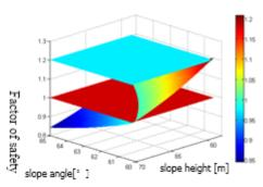
Fig. 11. 3D curve graphic revealing the relationship between factor of safety and slope heights and angles of typical section under the influence of three factors
