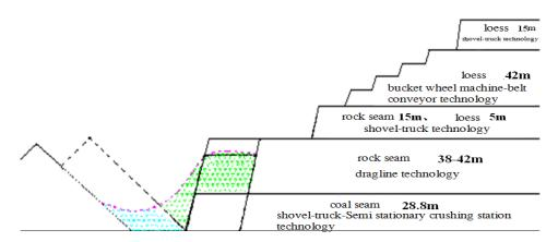
Fig. 3. Schematic diagram of mining technology section in West area
