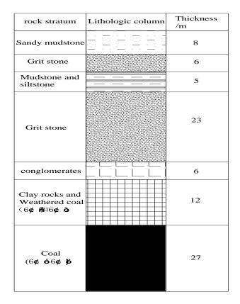
Fig. 4. Typical layers in Heidaigou Surface Mine
