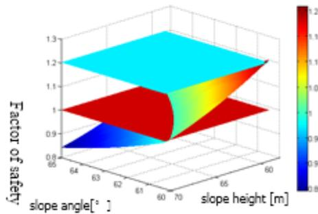
Fig. 11. 3D curve graphic revealing the relationship between factor of safety and slope heights and angles of typical section under the influence of three factors
