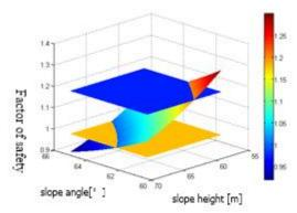
Fig.8. 3D curve graphic indicating the relationship between factor of safety, slope heights and angles with loading
