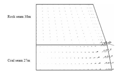
Fig. 14. Excavation to the 200m peak, the wedge changes in displacement plans
