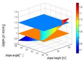
Fig.9. 3D curve graphic spitting the relationship between factor of safety, slope heights and angles with influence of blasting
