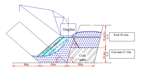
Fig. 1b. Sketch of dragline work on the high rock bench
