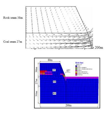
Fig. 13. x=165m failure graph digged
