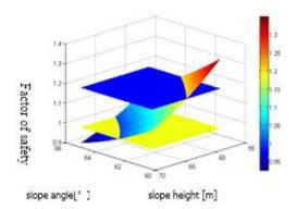
Fig.7. 3D curve graphic showing the relationship between factor of safety, slope heights and angles without loading
