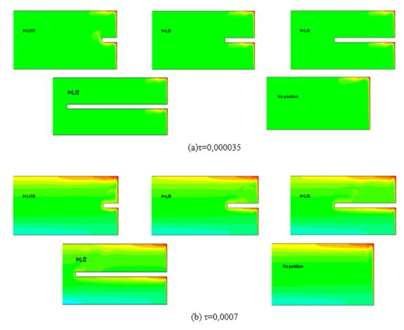
Fig.6. Thermal flows, (a) in the early stage, (b) in the quasi-steady stage, for different partitions length.
