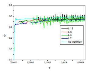
Fig.4. Temperature versus time, plotted at point (0.498, 0.09) for Ra = $3.77*10^9$  at different partition lengths
