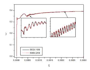
Fig.2. Temperature time series calculated by using different grids for the case of  $Ra = 3.77*10^9$ , and partition length of L/4. at the point (0.498,0.09) plotted.
