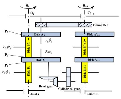
Fig.2. Structure Diagram of Joint i Mechanical System
