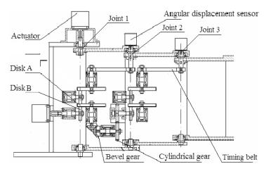
Fig. 3. Structural Diagram of Three Joints Nonholonomic Manipulator
