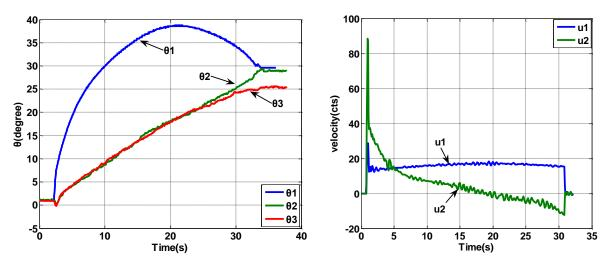
Fig.9. Joint Angles Displacement (Experiment) Fig.10. Input Angular Velocity (Experiment)
