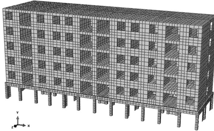
Fig.1. The 3D solid finite element model of 6-story masonry buildings
