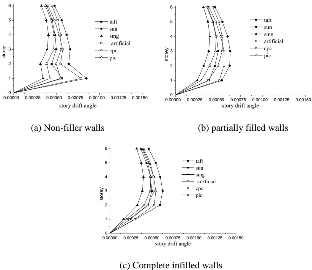
Fig.6. Story drift angle under Taft wave
