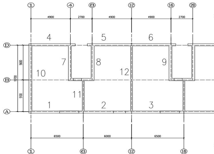
Fig.2. Building layout and filler wall arrangement diagram
