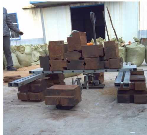
Figure 2: Elastic load stage the 0.2\text{m} \times 1\text{m} formwork
