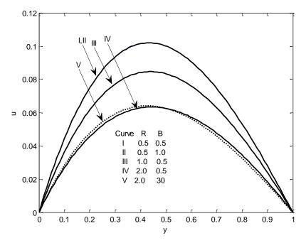
Fig 4: Velocity profiles showing effect of R, B (S = 0,  $K_c = 0$ ) for  $m = m_1 = 0$ .
