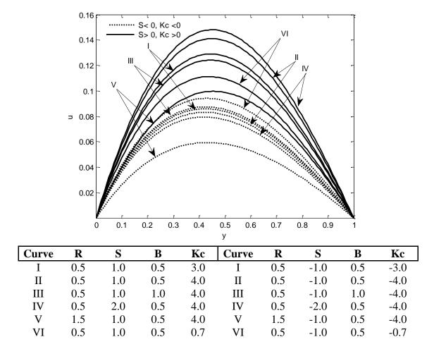
Fig 2: Velocity profiles showing effect of R, S, B ,  $K_c$  for  $m = m_1 = 0$  (asymmetric).
