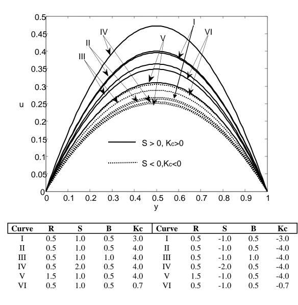
Fig 3: Velocity profiles showing effect of R, S, B,  $K_c$  for  $m = m_1 = 1$  (symmetric).
