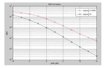
Figure 5. BER of SM based full duplex system performance
