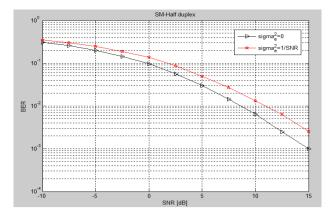
Figure 6. BER of SM based Half duplex system performance
