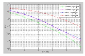
Figure 7. Comparison of QSM and SM System in FD and HD at  $Sigma_e^2 = 0$
