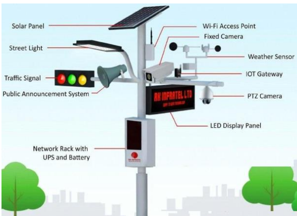
Figure 5. Smart electric poles equipped IoT gateway
