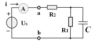
Fig.4. One Order RC Zero State Circuit
