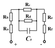
Fig.2. Electro-osmosis Equivalent Circuit Diagram
