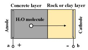
Fig.1. Electro-osmosis Arrangement Profile
