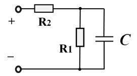
Fig.3. Equivalent Simplified Diagram of Electro-osmosis
