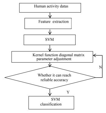
Fig.1. Asymmetrical SVM Detection Model
