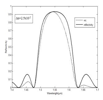
Fig.2. Reflectivity Profile with Wavelength for Raised-Cosine Apodized Function, and Compared with Ideal Relfective Profile
