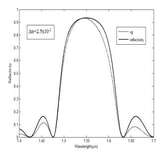
Fig.3. Reflectivity Profile with Wavelength for Gaussian Apodized Function, and Compared with Ideal Relfective Profile
