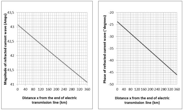
**Graph 2.** Magnitude (intensity) and phase (angle) of current refracted wave from the end towards the beginning of line ie. the direction the refracted wave moves (direction opposite to that of graph 1 ie. left to right of electric power transmission line of figure 1)
