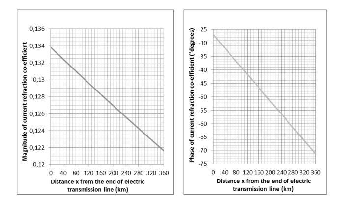
**Graph 3.** Magnitude and phase (angle) of current refraction co-efficient from the end where the refraction occurs towards the beginning of line (direction opposite to that of graph 1 ie. left to right of electric power transmission line of figure 1)
