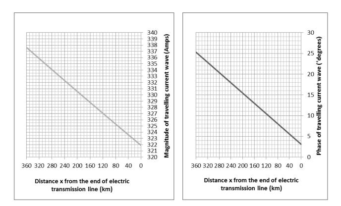
**Graph 1.** Magnitude (intensity) and phase (angle) of current travelling wave from the beginning towards the end of line ie. the direction the travelling wave moves (direction right to left of electric power transmission line of figure 1)
