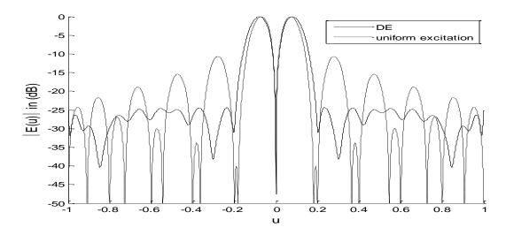
Fig. 7. Patterns for DE optimized and uniformly excited arrays
