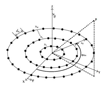
Fig. 2.Geometry of concentric circular array
