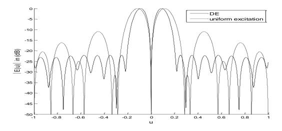
Fig. 3. Patterns for DE optimized and uniformly excited arrays
