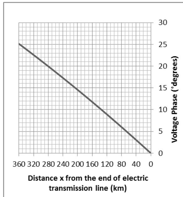
**Graph 2.** Voltage magnitude (left graph) and voltage phase (angle) (right graph) from the beginning towards the end of line (direction opposite to that of
