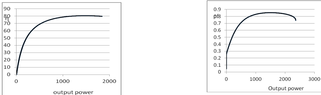
Fig. 2 Performance characteristics of designed three phase squirrel cage induction motor
